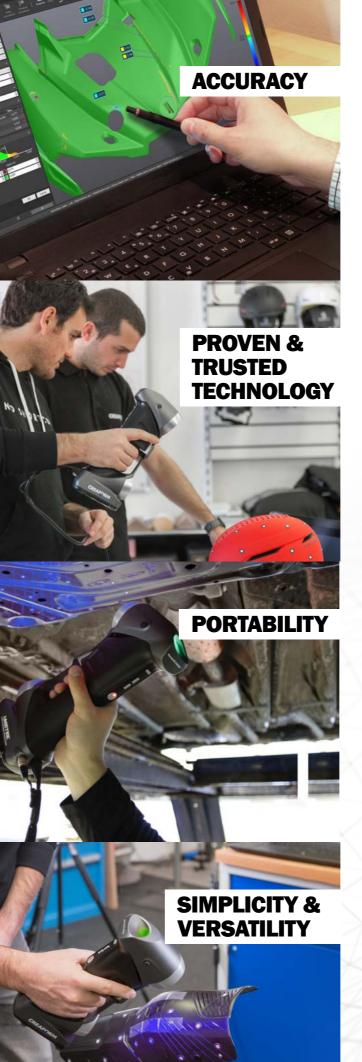
The HandySCAN 3D | SILVER Series delivers accurate and reliable 3D measurements regardless of the measurement setup quality and the user's experience level. Featuring dynamic referencing, both the scanner and part can move freely during scanning, and an accurate and high quality scan can still be obtained.
